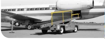
Replacement Safety Rail is designed to retrofit onto TUG 660 Belt Loaders. It features an adjustable angle reduced height handrail at the aircraft end of the belt to clear the engine cowl of regional jets.
