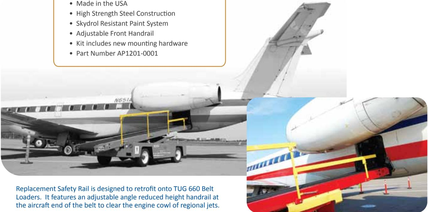
Replacement Safety Rail is designed to retrofit onto TUG 660 Belt Loaders. It features an adjustable angle reduced height handrail at the aircraft end of the belt to clear the engine cowl of regional jets.
